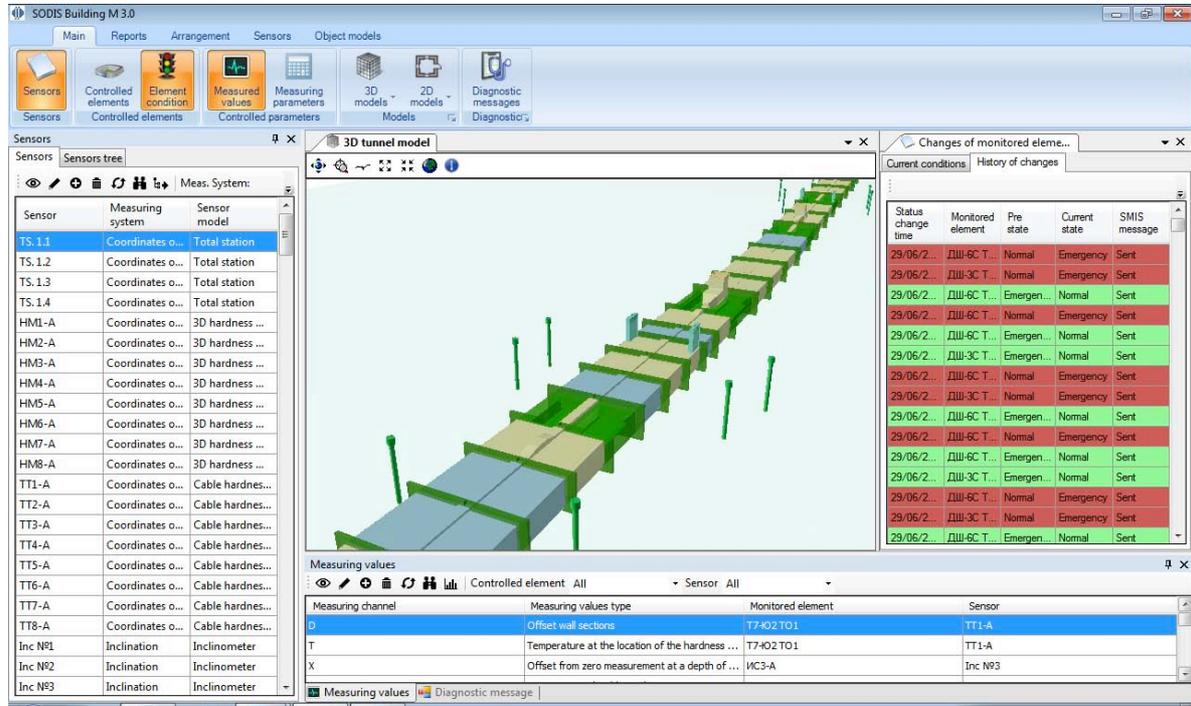
Figure 4: SODIS Building M software screen for building operators
