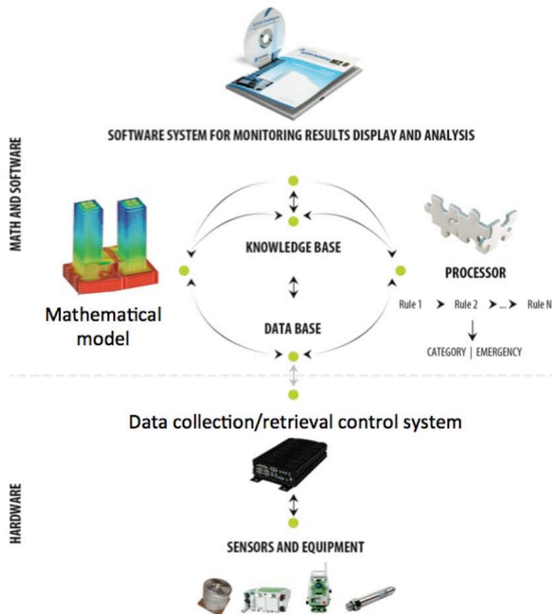
**Figure 2:** Structural monitoring system architecture
