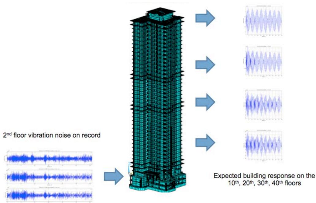
**Figure 6:** Model verification by inputting 2<sup>nd</sup> floor noise record to the mathematical model
